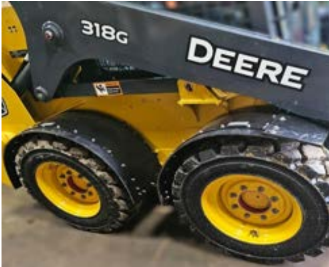
Figure 2: D-Fender Inside Diameter
